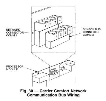
NOTE: Conductors and drain wire must be 20 AWG (American Wire Gage) minimum stranded, tinned copper. Individual conductors must be insulated with PVC, PVC/nylon, vinyl, Teflon, or polyethylene. An aluminum/ polyester 100% foil shield and an outer jacket of PVC, PVC/ nylon, chrome vinyl, or Teflon with a minimum operating temperature range of -4 F to 140 F (-20 C to 60 C) is required. See table below for cables that meet the requirements.
